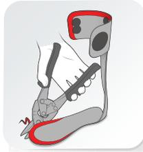
Using industrial tin snips or a dremel saw, trim the footplate to the template size and do not trim beyond red section
